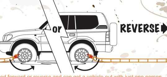
BOG OUT can be used forward or reverse and can get a vehicle out with just one person.
