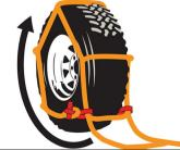
Attach other end of **BOG OUT** to a suitable anchor point and drive **SLOWLY** out of bog.
